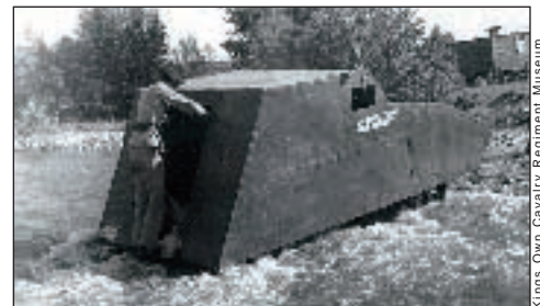
A mock tank—a Model-T Ford with a canvas superstructure—created by the Calgary Regiment (Tank) for training in 1938.
