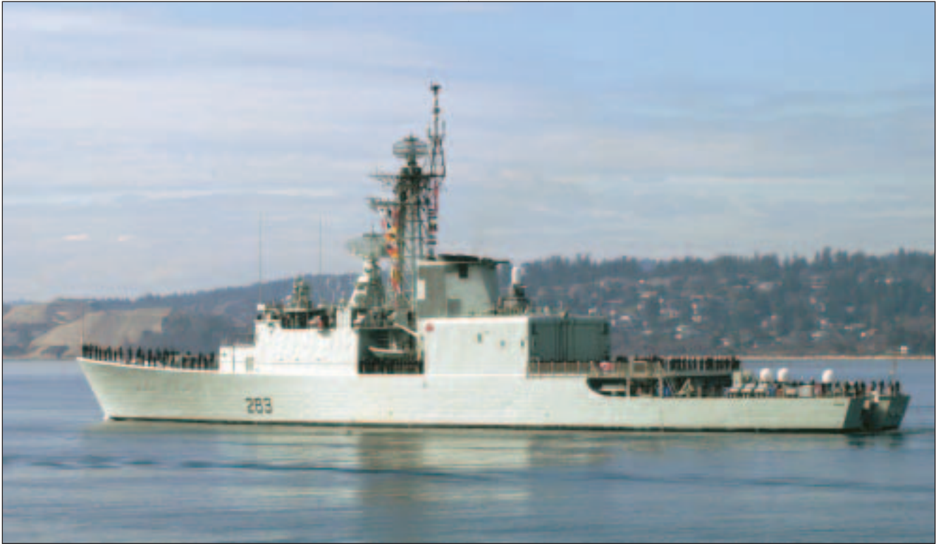
As a further example of a host platform for EW jamming/deception systems employed in recent decades, the Canadian destroyer HMCS Algonquin carries the SLQ-501 Canadian Naval Electronic Warfare System (CANEWS), the SLQ-503 jammer and the SLQ-25 Nixie torpedo deception system, as well as four 6-barrelled Plessy Shield IR /chaff dispensers and the Nulka hovering decoy system.
