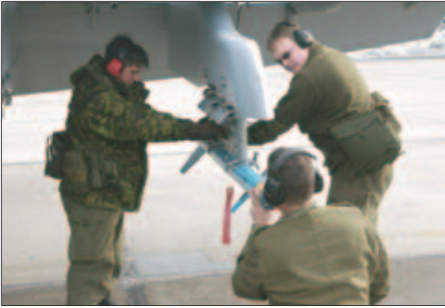
No room for debate here. Armament technicians load a Laser Guided Training Round (LGTR) to a 441 Squadron CF-18 Hornet on the hangar line at 4 Wing Cold Lake.
