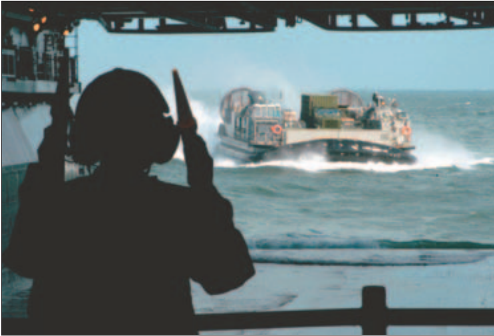
Another shot of a LCAC being directed into the well deck of the USS Iwo Jima as it steams toward the Gulf Coast in August 2005.
