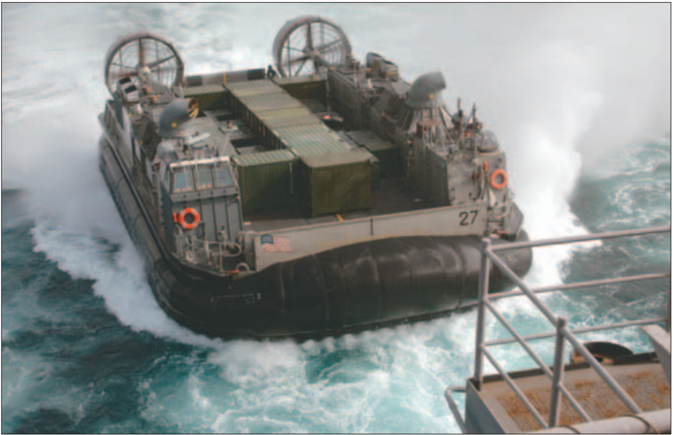
A U.S. Navy Landing Craft Air Cushion (LCAC) manoeuvres to enter the well deck of the amphibious assault ship USS Kearsarge in June 2005.
